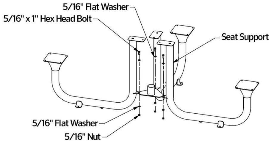
5. Position the remaining seat support so that it aligns with the remaining mounting hole in the lower leg bracket. Attach the seat support to the lower leg bracket using a 5/16" x 1" hex head bolt with 5/16" flat washers on the top and bottom and a 5/16" Nylock nut to secure. Leave the hardware finger tight until after the table top pan is secured (step 7).
