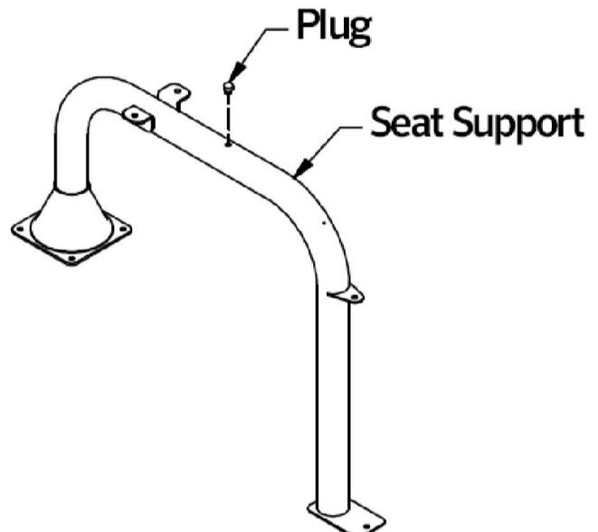
4. Locate two seat supports and the lower leg bracket. Position the seat supports so that they will be opposite each other when fastened to the lower leg bracket. Install 5/16" flat washers on 5/16" x 1" hex head bolts and insert the bolts through the appropriate mounting holes in the lower leg bracket and into the lower mounting holes in the seat supports. Place 5/16" flat washers and 5/16" Nylock nuts on the end of the bolts and tighten finger tight.
