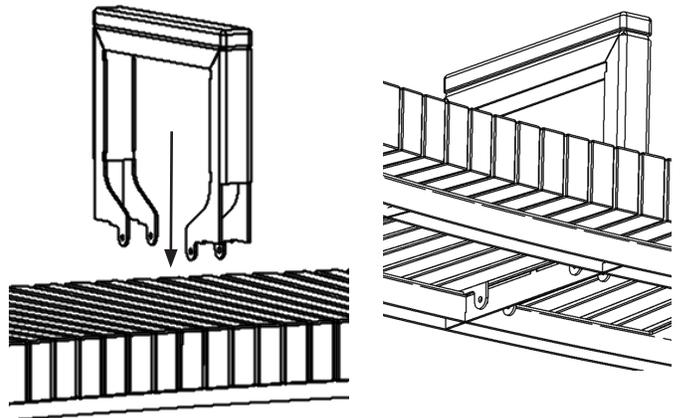
2. Locate under bracket and insert the threaded ends of the u-bolts through the slots in the bottom and attach the 1/4"-20 nuts provided loosely.
