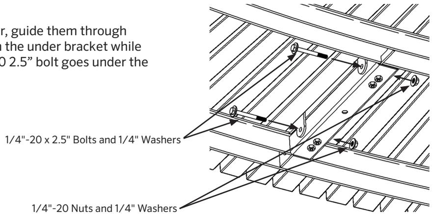
5. Secure the bolts with 1/4"-20 nuts and washers tighten finger tight.
