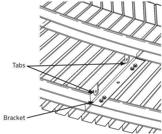
4. Locate a 1/4"-20 x 2.5" bolt and washer, guide them through the holes in the armrest and the slot on the under bracket while pushing up on the u-bolt so the 1/4"-20 2.5" bolt goes under the u-bolt. Repeat for the other side.
