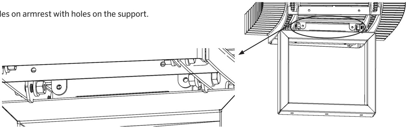
3. Insert two 1/4"-20 x 2.5" bolts with washers through armrest and support.
