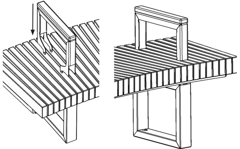
2. Align holes on armrest with holes on the support.
