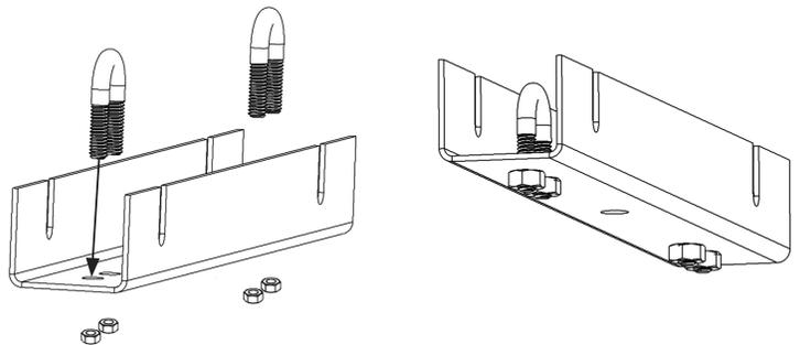
3. On the underside of the bench, slide the under bracket in between the tabs of the armrest and slide the bracket up until it makes contact with the under support of the bench.
