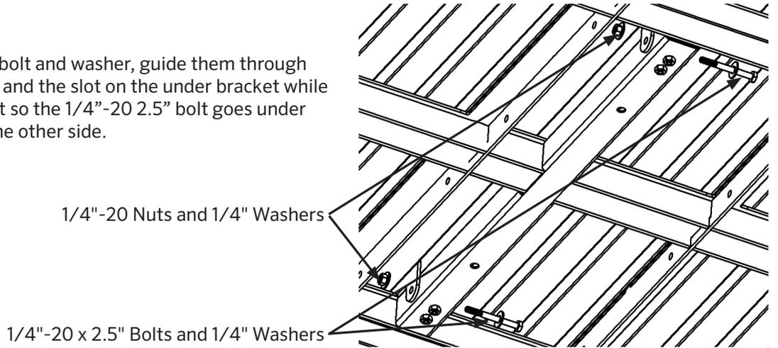
5. Secure the bolts with 1/4"-20 nuts and washers tighten finger tight.
