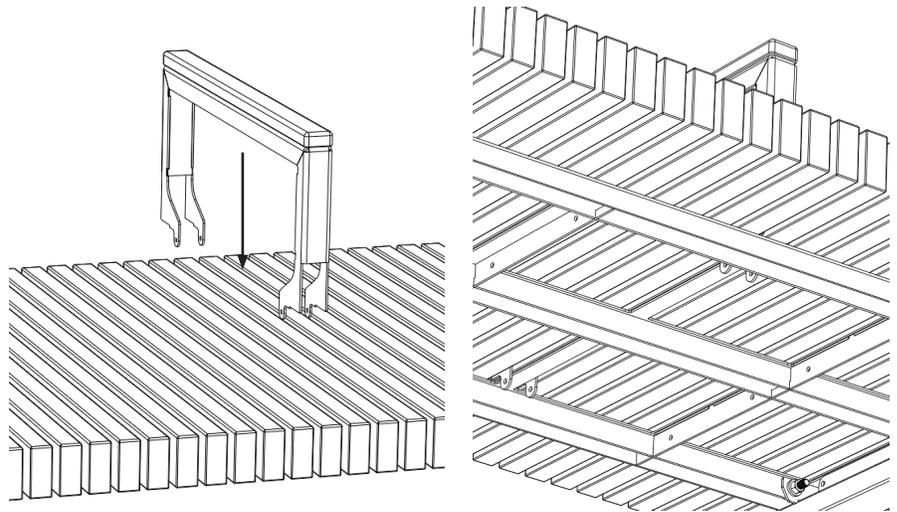
2. Locate under bracket and insert the threaded ends of the u-bolts through the holes in the bottom and attach the 1/4"-20 nuts provided loosely.
