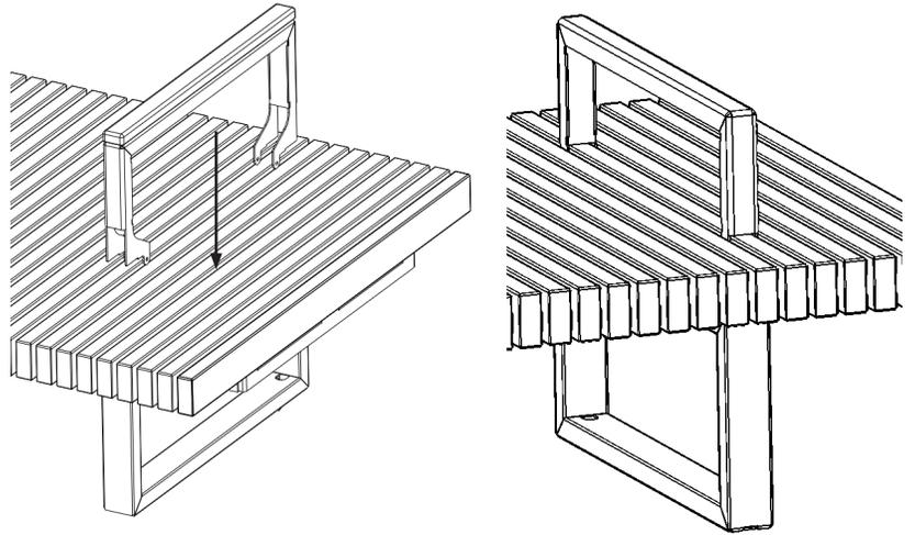
2. Align holes on armrest with holes on the support. Insert two 1/4"-20 x 2.5" bolts with washers through armrest and support.
