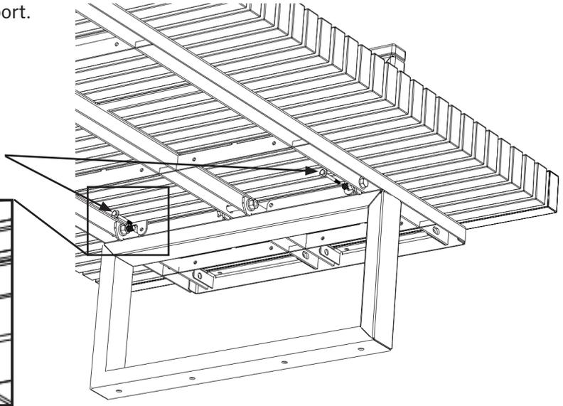
3. Place a 1/4"-20 nut and a 1/4" washer onto each of the bolts and tighten finger tight.
