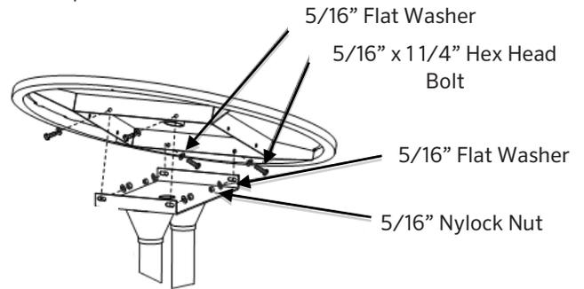
Leave the bolts finger tight until all the Nylock nuts are started. Then use the 1/2" open end or box end wrench and ratchet with the 1/2" socket to tighten the hardware.
