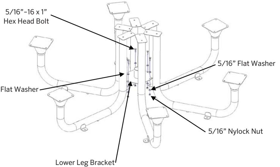
5. Repeat step 4 for the remaining seat supports. Leave the hardware finger tight until after the table top pan is secured.
