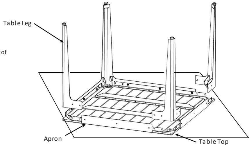
5. Insert one 1/4" flat washer and one 1/4" Nylock nut per each PEM® stud.
