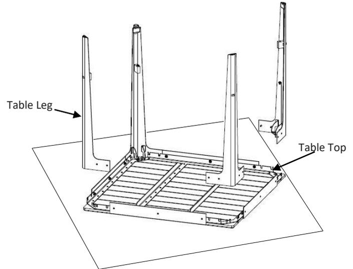
5. Insert one 1/4" flat washer per each PEM® stud. Then screw on a 1/4" Nylock nut and loosely hand-tighten all four legs.
