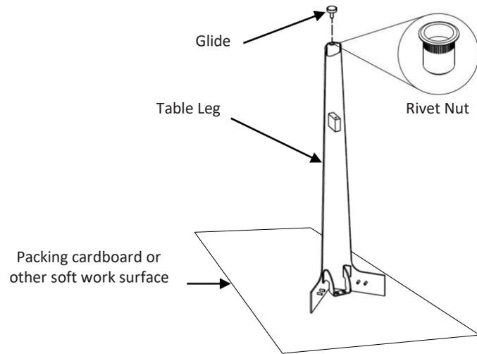
4. While leaving the pre-assembled table top upside down on the padded work area, slide each leg down the slots of each corner of the table top as shown.
