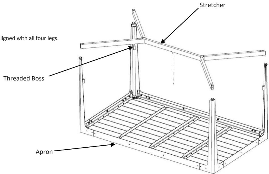
7. Place one 1/4" flat washer onto one 1/4"-20 x 1/2" button head socket cap screw. Then insert the screw into the threaded boss as shown.
