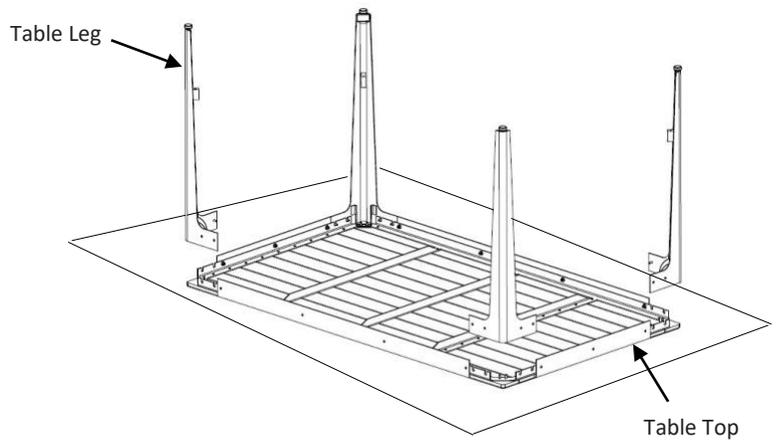
5. Insert one 1/4" flat washer per each PEM® stud. Then screw on a 1/4" Nylock nut and loosely hand-tighten all four legs.
