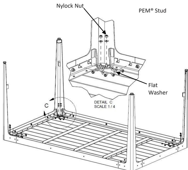
6. Slide the stretcher into place making sure it's aligned with all four legs.
